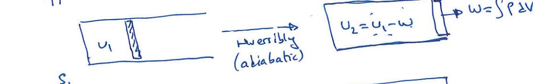
$$U_2 = U_1 \left( \frac{V_1}{V_2} \right)^{2/3}$$
