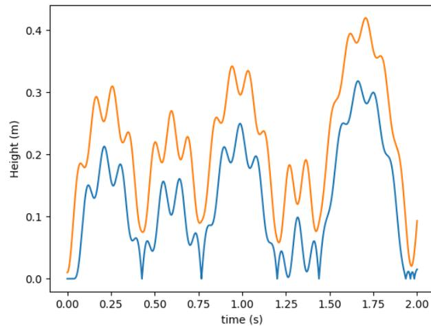
Figure 1: The positions of the masses as a function of time. Notice that the lower curve (corresponding to  $y_1$ ) hits  $y_1 = 0$  every once in a while.
