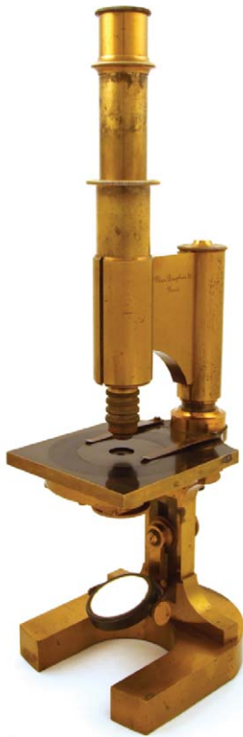
Figure 2 Microscope stand VIII, No. 4815 manufactured by Hartnack successor of Oberhaeuser in Paris, France, in 1864. This is the first microscope stand to show the horse-shoe base. All photos © by Timo Mappes, Karlsruhe (www.musoptin.com) and reproduced by permission.
