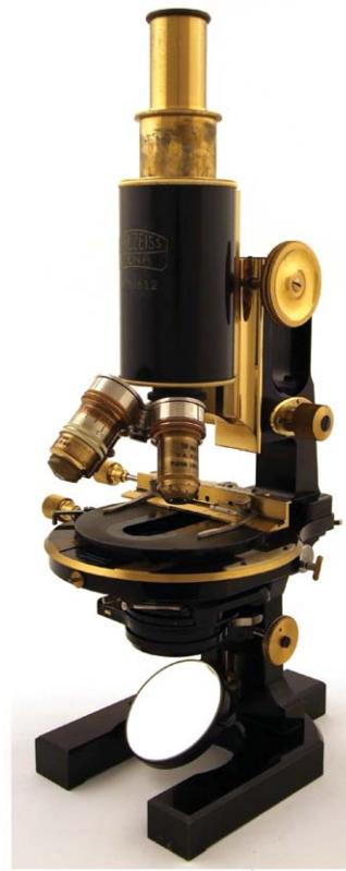
Figure 5 Microscope stand I e , No. 51612 manufactured by Carl Zeiss, Jena, Germany, in 1910. The microscope stand is called the 'jug handle' stand and was made from 1898 to 1920 and was copied by other microscope manufacturers. The particular microscope shown is equipped with Zeiss apochromats and is the personal instrument of Raymond-Joseph Weissenbach (1885–1963), who gave the name to the Thibièrge-Weissenbach syndrome. All photos © by Timo Mappes, Karlsruhe (www.musoptin.com) and reproduced by permission.
