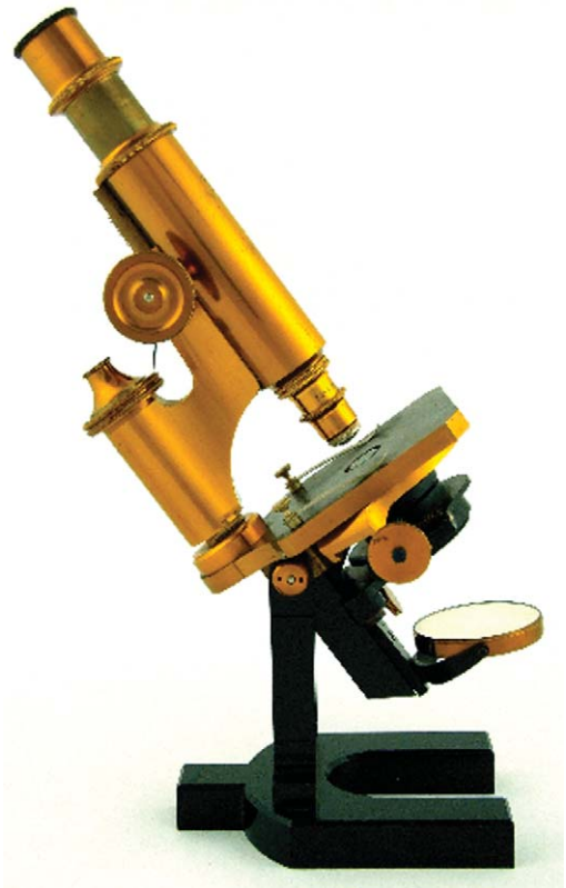
Figure 3 Microscope stand II, No. 5272 manufactured by Carl Zeiss, Jena, Germany, in 1881. It is equipped with an Abbe condenser and a homogeneous immersion objective. Santiago Ramón y Cajal (Spain) and Robert Koch (Germany) used this type of microscope. All photos © by Timo Mappes, Karlsruhe (www.musoptin.com) and reproduced by permission.
