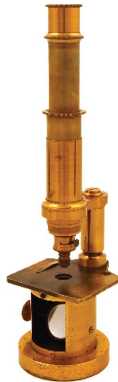
Figure 1 Microscope stand IV, No. 3207 manufactured by Oberhaeuser and Hartnack in Paris, France, in 1858. This microscope has a drum stand and polarizing equipment. This type of microscope was used by Rudolf Virchow in Berlin, Germany. All photos © by Timo Mappes, Karlsruhe (www.musoptin.com) and reproduced by permission.
