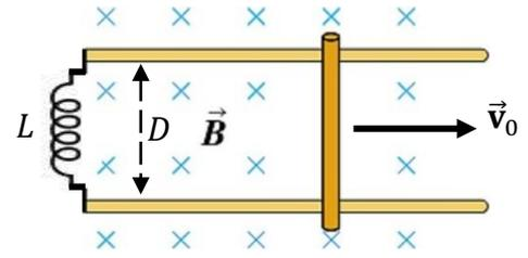
**Solution:** (a) If  $v(t)$  is the speed of the bar at time  $t$ , then  $\mathcal{E}(t) = BDv(t)$  is the motional emf induced at the two ends of the rod. This is also equal to the voltage across the inductor. So
