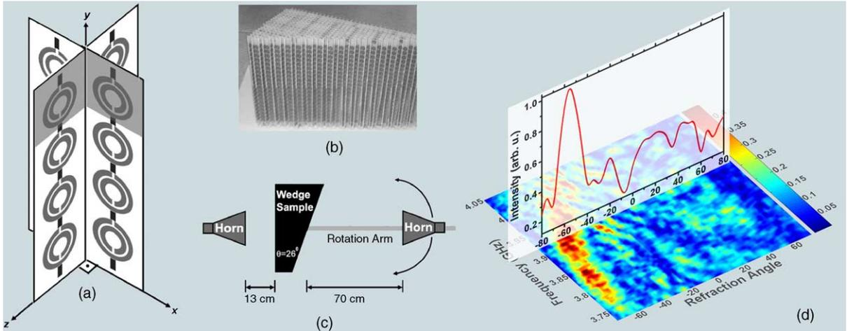
Fig. 3. (a) The unit cell (shaded) of the 2D CMM. (b) Actual photo of the 2D CMM prism with  $\theta_t = 26^\circ$  apex angle. (c) Schematic of the experimental set-up. (d) The angular refraction spectrum. The light shaded band around  $-60^\circ$  denotes higher intensity. The angular cross-section at  $f = 3.92$  GHz yields a refractive index  $-1.87 \pm 0.05$ .
