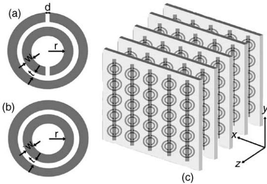
Fig. 1. The schematic representation of (a) SRR, (b) CRR, and (c) CMM structures. The parameters are  $d = t = 0.2$  mm,  $w = 0.9$  mm,  $r = 1.6$  mm. Wire thickness is  $w = 0.9$  mm. The unit cell has dimensions  $a_x = a_y = 8.8$  mm and  $a_z = 6.5$  mm.
