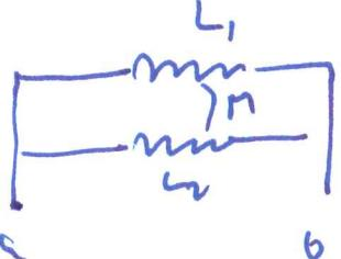
$$\rightarrow V_{ab} = d L_1 \frac{dI_1}{dt} + M \frac{dI_2}{dt} \\ = L_1 \frac{dI_2}{dt} + M \frac{dI_1}{dt} = L_{eq} \frac{dI}{dt}$$
