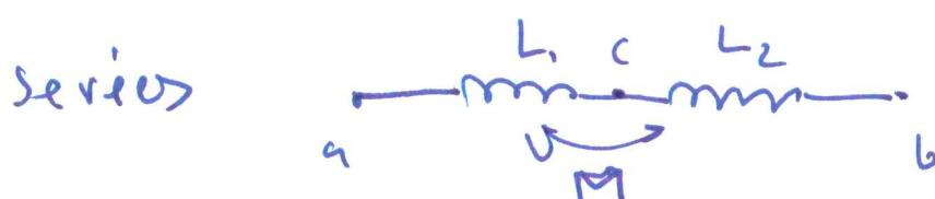
$$V_{ac} = L_1 \frac{dI}{dt} + M \frac{dI}{dt}$$
