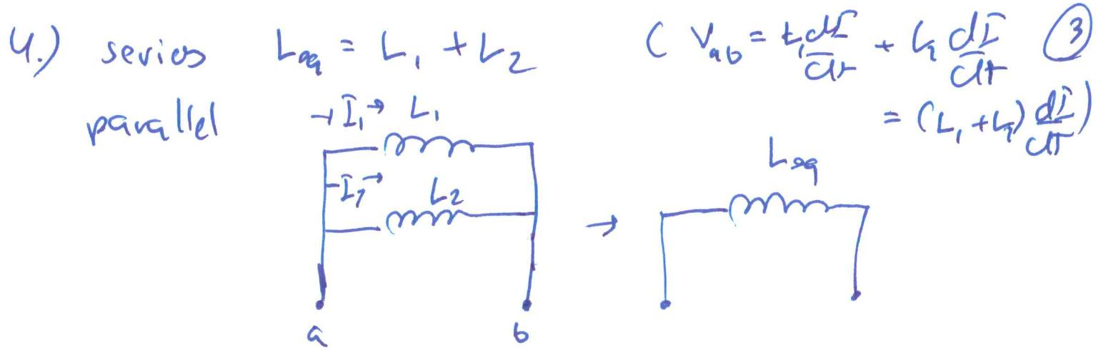
$$V_{ab} = L_{eq} \frac{dI}{dt} = L_1 \frac{dI_1}{dt} = L_2 \frac{dI_2}{dt} \Rightarrow \frac{dI}{dt} = \frac{dI_1}{dt} + \frac{dI_2}{dt}$$
