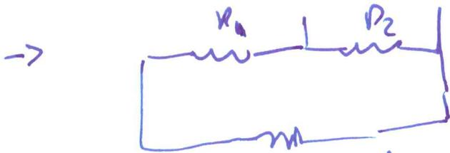
$$R'' = \frac{R_2 R_3}{R_2 + R_3} = 23.3 \Omega$$
