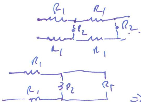
$$R_T = 2R_1 + \frac{R_2 R_T}{R_1 + R_T}$$
