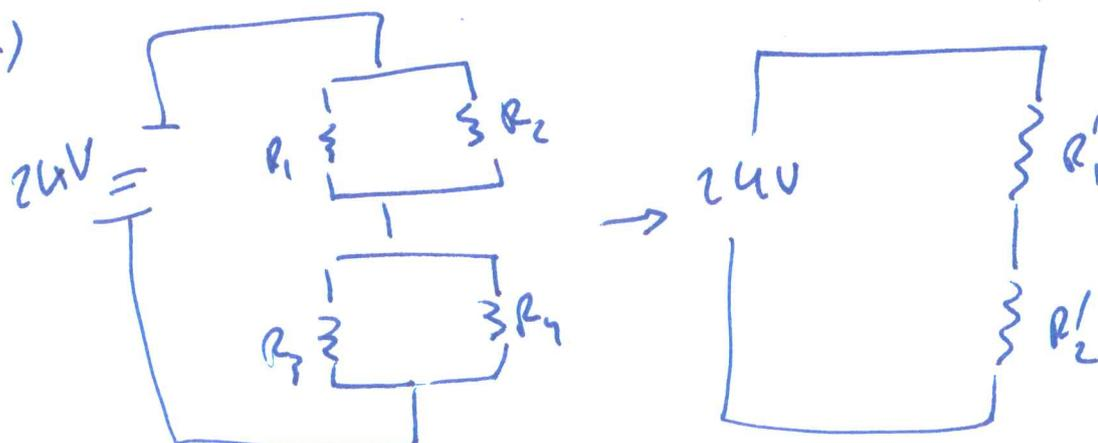
$$R_1' = \frac{R_1 R_2}{R_1 + R_2} \quad R_2' = \frac{R_3 R_4}{R_3 + R_4}$$
