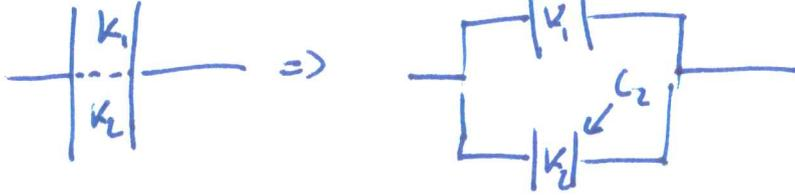
capacitance:  $C_{eq} = C_1 + C_2$
