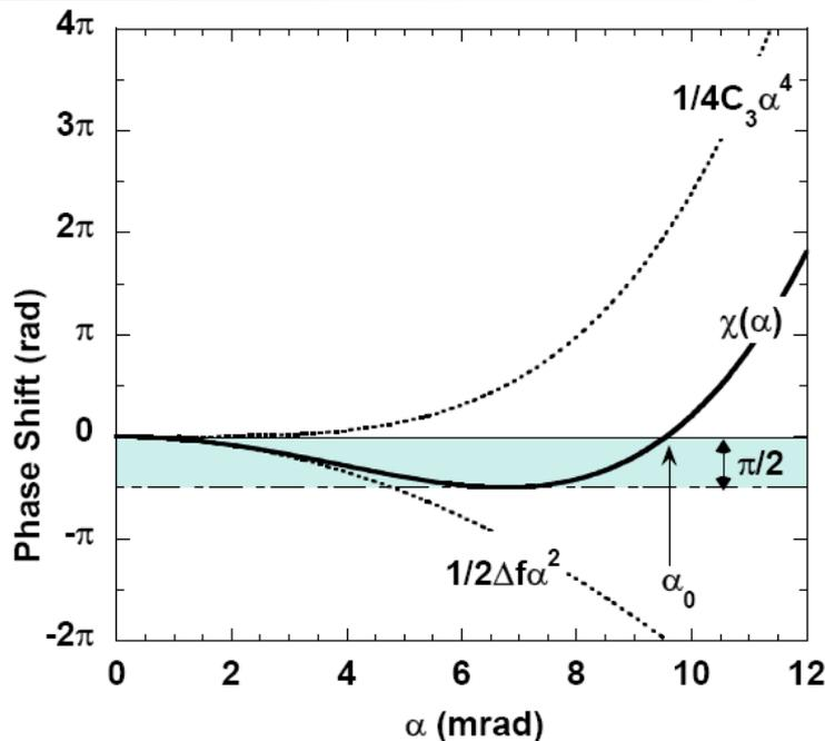
Step 1: Pick largest tolerable phase shift: in EM  $\lambda/4 = \pi/2$ , in light optics  $\lambda/10$
