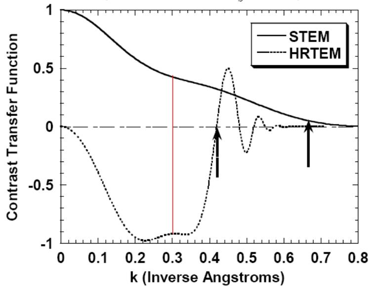
TEM: Bandpass filter: low frequencies removed = artificial sharpening
