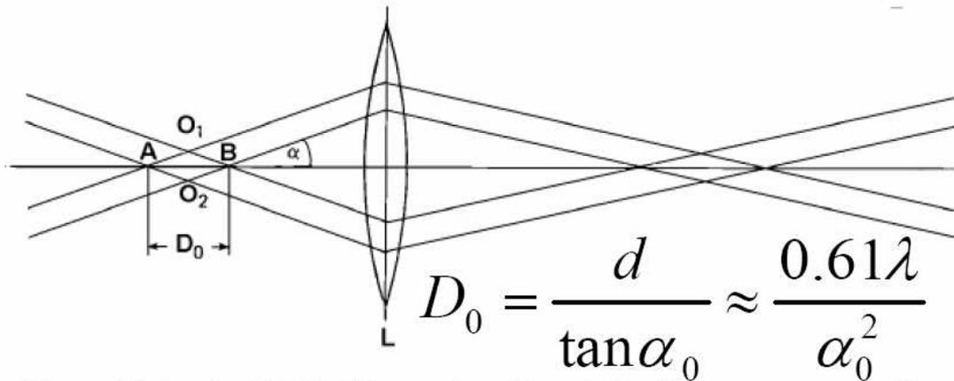
**Figure 11. Depth of field.** Object points  $O_1$  and  $O_2$  objects are separated by the resolution limit  $d$  of the lens. Rays from these points cross the axis at  $A$  and  $B$  equally. Hence, points between  $A$  and  $B$  will look equally sharp, and  $AB$  is the depth of field  $D_0$  of the lens for a semi-angular aperture  $\alpha$ .
