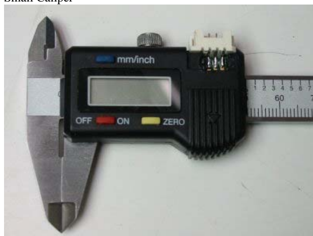
Connector soldered to caliper PCB - 2.0mm Hirose DF-3 series SMT right angle - DigiKey H2129-ND
