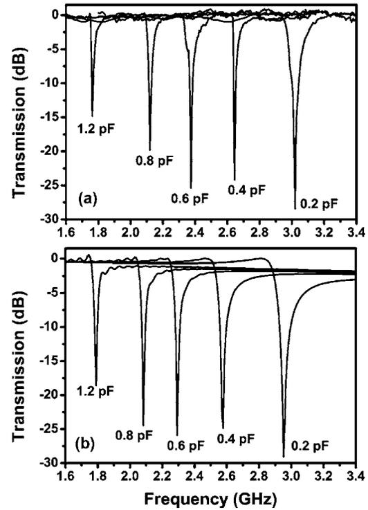
FIG. 5. Transmission coefficients of SRR structures with capacitors loaded at the inner split region: (a) experimental data and (b) numerical simulations.
